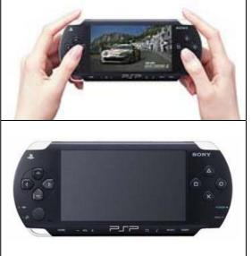
**PSP features** (see figures above): 333 Mhz processor, 32 Mb RAM, UMD-disk (mini-DVD): 1,8 GB, MPEG 4, Stereo Sound, HighRes 10 cm Screen, WIFI, USB 2.0, 5hrs Accu.,
