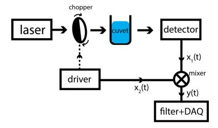
The chopper rotates at a certain frequency, such that the laser is blocked for half a period during each rotation of the chopper. The chopper is driven by a signal generator at a certain frequency  $f_1$ . The driver will also send a signal  $x_2(t) = \cos(2\pi f_1 t)$  to a mixer, which is used after the detected signal to down convert the signal back to DC, after which it is filtered and averaged.
