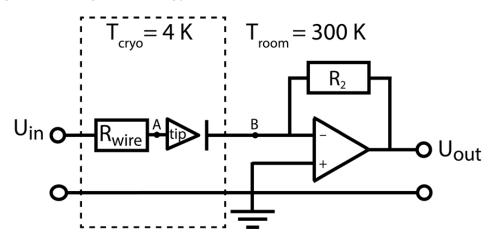
We are interested in the sources of noise of a Scanning Tunnelling Microscope. A voltage  $U_{in}=10~mV$  is applied between a metallic tip and a metallic surface, resulting in a tunnelling current I(t). We can model the system as a small wire resistance  $R_{wire}=1~\Omega$  in series with a vacuum resistance  $R_{vacuum}=10~G\Omega$ , all placed at a cryogenic temperature of 4 Kelvin.
