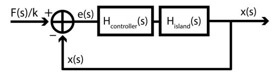
We can model a measurement island as a mechanical resonator. The differential equation for the motion x(t) of a mechanical resonator is given by:
