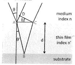
We start by calculating the optical path difference x between the beam that is reflected at the interface between the medium and the thin film (point A) and the beam that passes through the thin film and is reflected at the interface to the substrate (point B). This difference is given by
